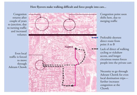
**FIGURE 19.4** How People are Forced to Use Motorized Vehicles for Short-distance Trips—Ashram Chowk Flyover, New Delhi *Source*: Solving Congestion through Transit Oriented Development, Romi Roy 2009.
